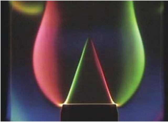
The flame front in a steady flow in a laboratory burner (left) contrasts with the distorted instantaneous flame front during an oscillatory flow.
